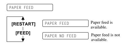
After selecting the paper feed, press the **[PAUSE]** key. The display returns to the "<4>TEST PRINT".
